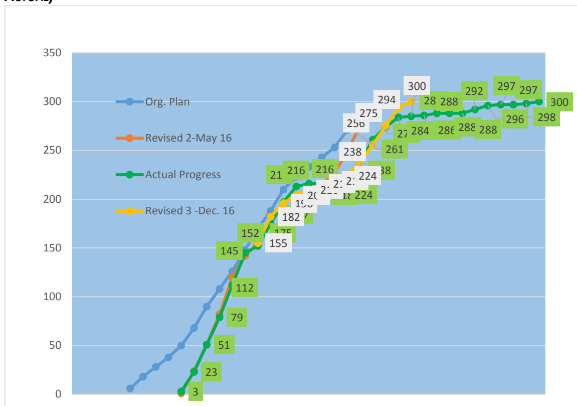
FIGURE 2-5: CUMULATIVE WORK PROGRESS OF TOWER FOUNDATION (ORIGINAL/REVISED PLANNED AND ACTUAL)
